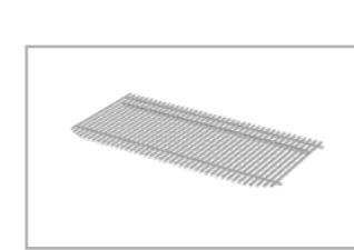
Remove the drip grid from the residual water tray and clean it.
