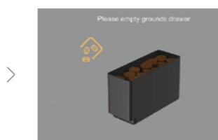
Remove, empty, clean and reinsert the grounds container. After that, press the arrow key to go to the next step.
