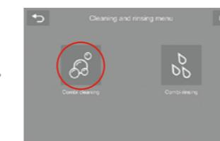
Press the COMBI-CLEANING button to start cleaning.
